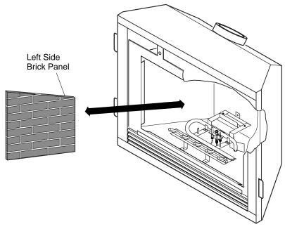
Figure 48 - Installing Left Side Brick Panel
